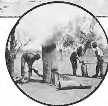
Hollow Tree Butt as a Native Forge
